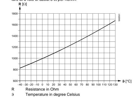
The sensing element is a nickel thin-film element having a basic resistance of 1000  $\Omega$  at 0 °C. The resistance of the element increases in function of the temperature at a rate of about 5  $\Omega$  per Kelvin.
