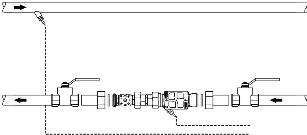
As an alternative, the sensors can be immersed directly in off-the-shelf ball valves with integrated measuring points (e.g. Siemens WZT-K.. / Jumo 902442/11) or t-pieces (e.g. Jumo 902442/31).
