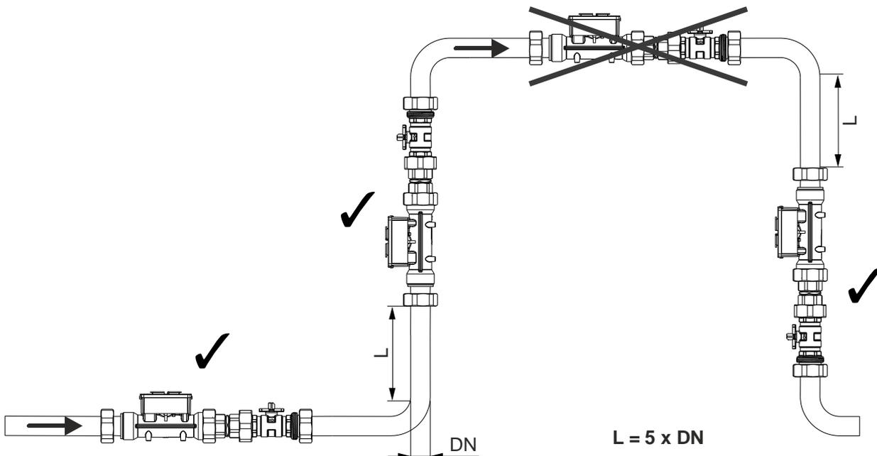
The rule is: Measure first, then control – in other words, the flow sensor must always be mounted upstream of the control valve in a compact installation.
