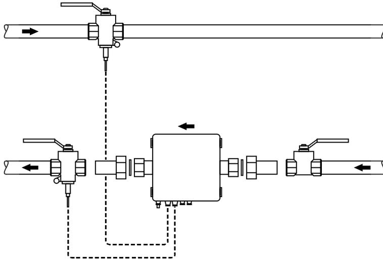
The brass protective pockets EZT-M40 are available for mounting with protective pockets.
