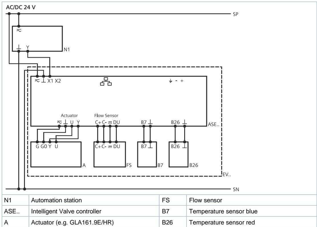
**For the control functions “Dynamic control valve” and “Dynamic control valve (changeover)” – Setpoint source Modbus**
